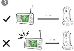
To avoid interference from other electronic devices, place your baby monitor at least 1 metre away from devices such as wireless routers, microwaves, mobile phones and computers.
