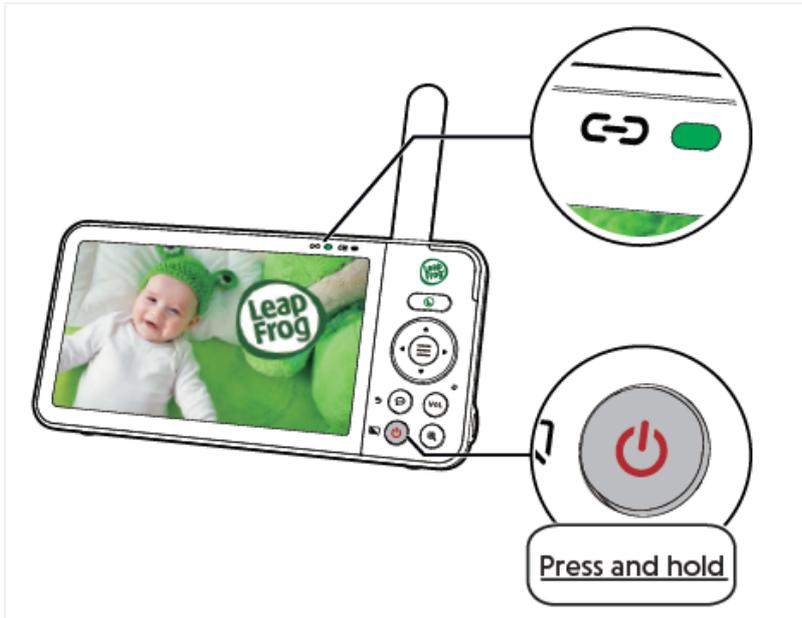
3. Once your Baby Unit and Parent Unit are powered on, your Parent Unit displays image from the Baby Unit, and the **LINK LED** light turns on. The Baby Unit's **POWER LED** light also turns on.
