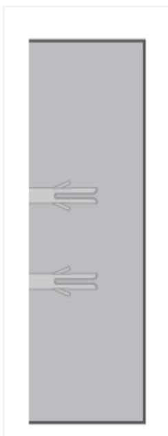
3. Insert the screws into the holes and tighten the screws until only 6.5 mm of the screws are exposed.
